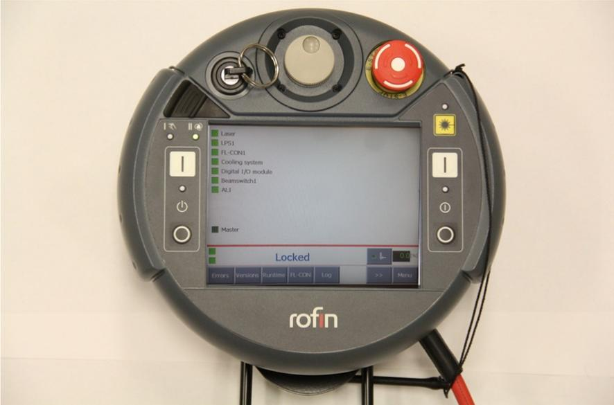
Figure 38: This screen provides an overview of the laser status and will help in troubleshooting errors and faults. This is also the screen where a user can **enable master**, the first step in changing the **program mode**.
