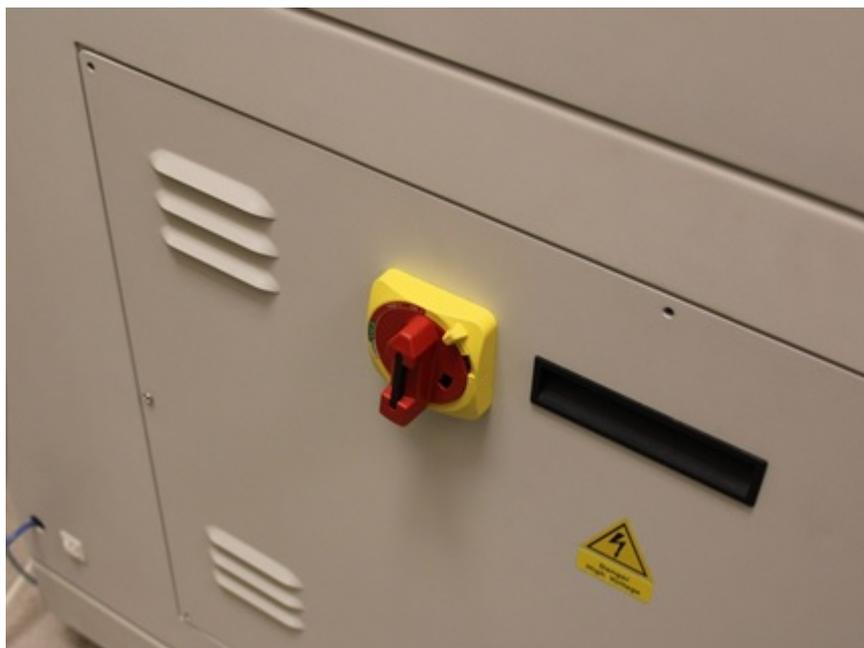
Figure 6: Workstation main power disconnect.
