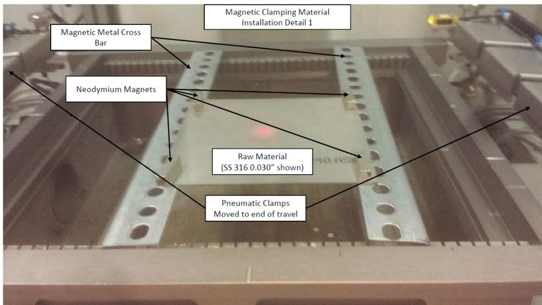
Figure 25: Move the pneumatic clamps to the end of their travel and secure them. Install the **magnetic metal cross bars** in the cutting box so that the raw material ends rest upon them. Using the Neodymium magnets located on the cabinet adjacent to the workstation on the right, secure the raw material edges. Add **material support bars** as needed to provide support interior to the material edges.
