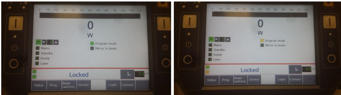
Figure 10: Menu screen for VLM (left) and Internal Programs (right) operating modes.
