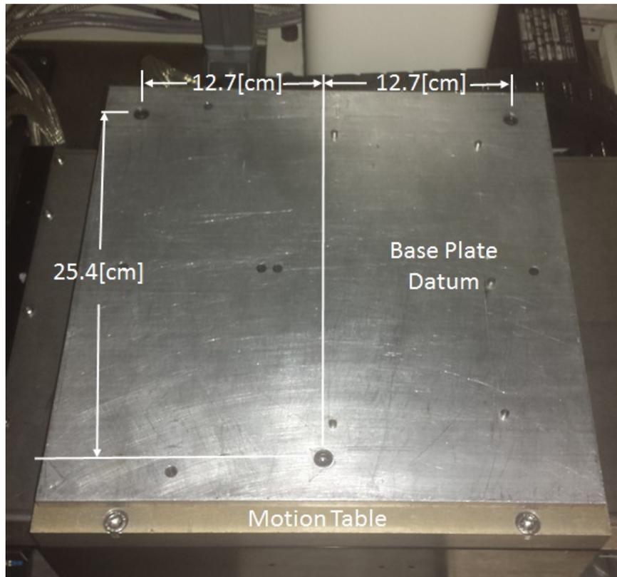
Figure 34: A typical base-plate datum made of 6061 Aluminum used for stainless steel and superalloy welding. Aluminum has a high thermal conductivity which prevents welded parts from sticking to the base plate. **NOTE:** Three holes with a diameter of 0.245[in] are required for mounting a plate on the stage. The bolt pattern is shown.
