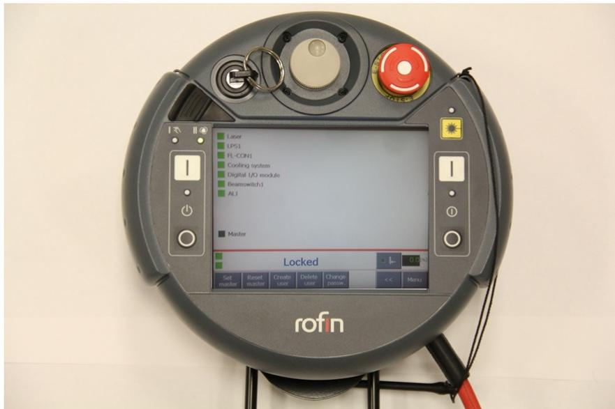
Figure 44: The additional options on the **status** screen that are revealed after selecting the **double-right arrow** button.
