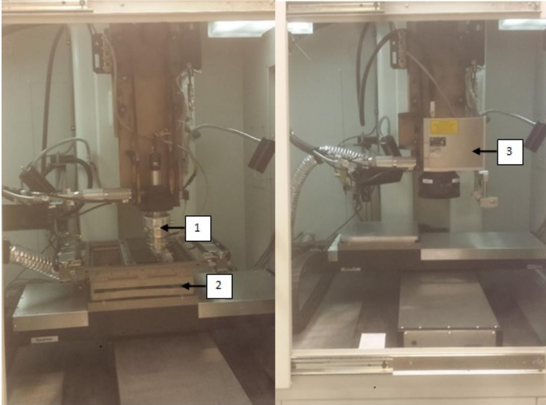
Figure 2: Cutting(Left) and Welding(Right) Optics installed on workstation z-axis.
