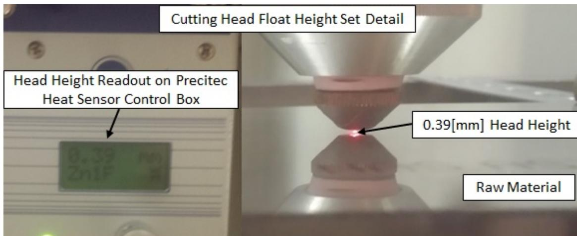
Figure 27: Cutting height properly set showing Precitec readout(left) and optics(right).
