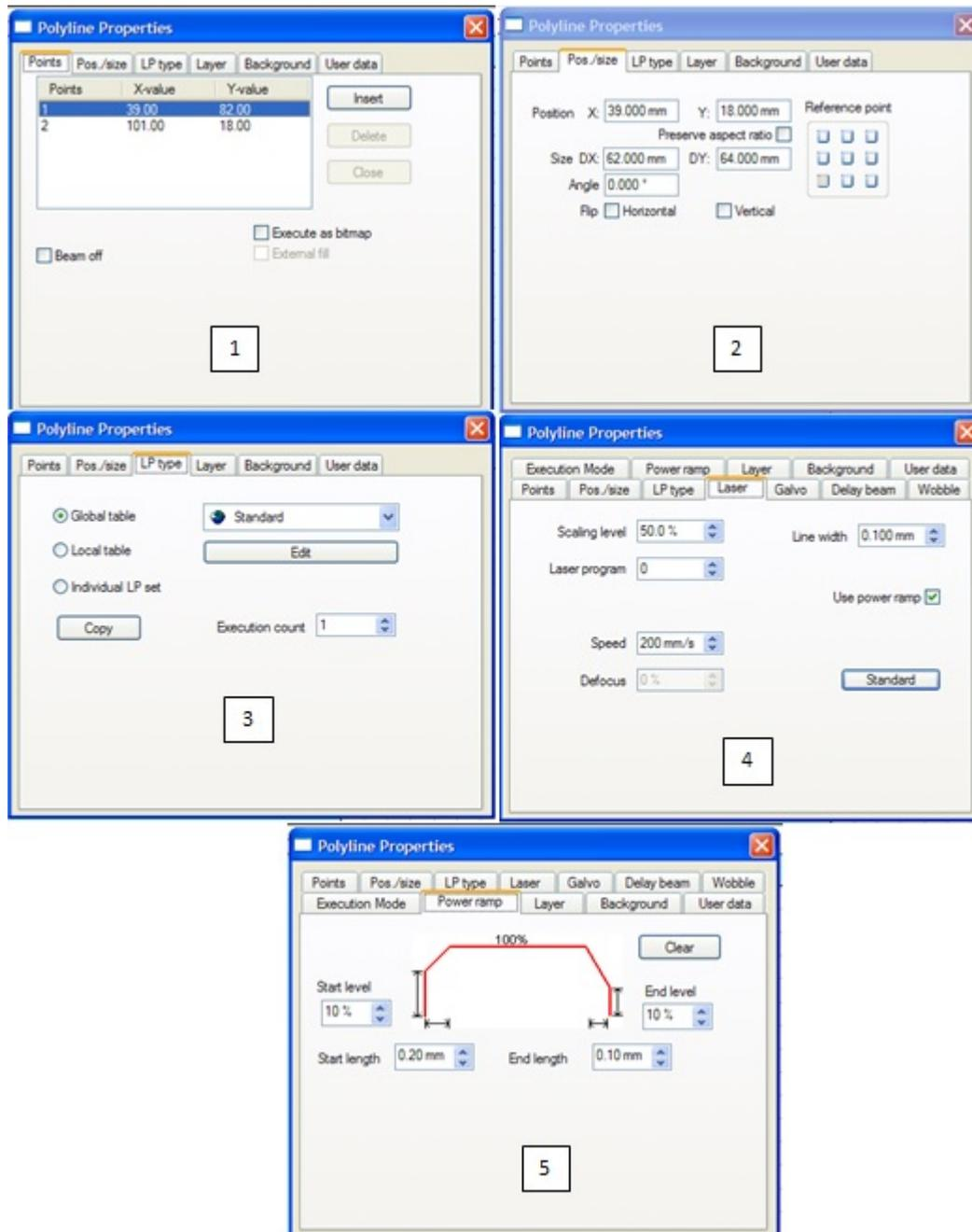
Figure 54: 5 useful properties pages for a drawing element. Access these properties by double-clicking on the drawing element you wish to change to properties of.
