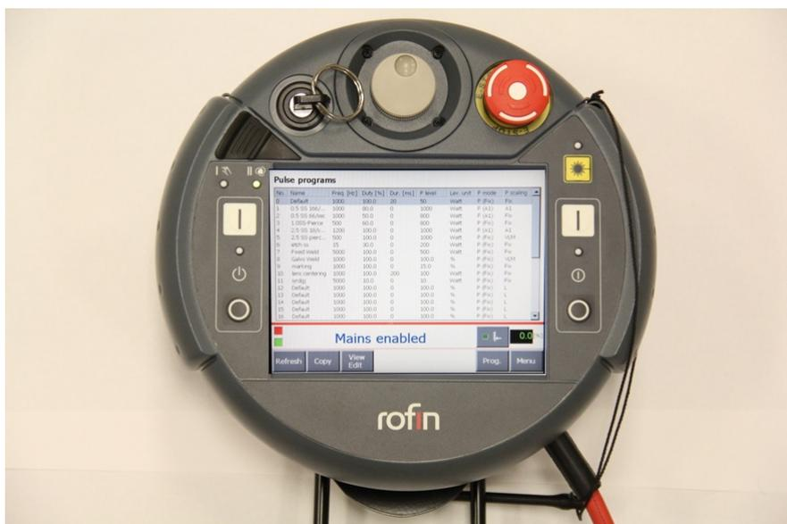
Figure 40: This screen provides an overview of all pulse programs available.
