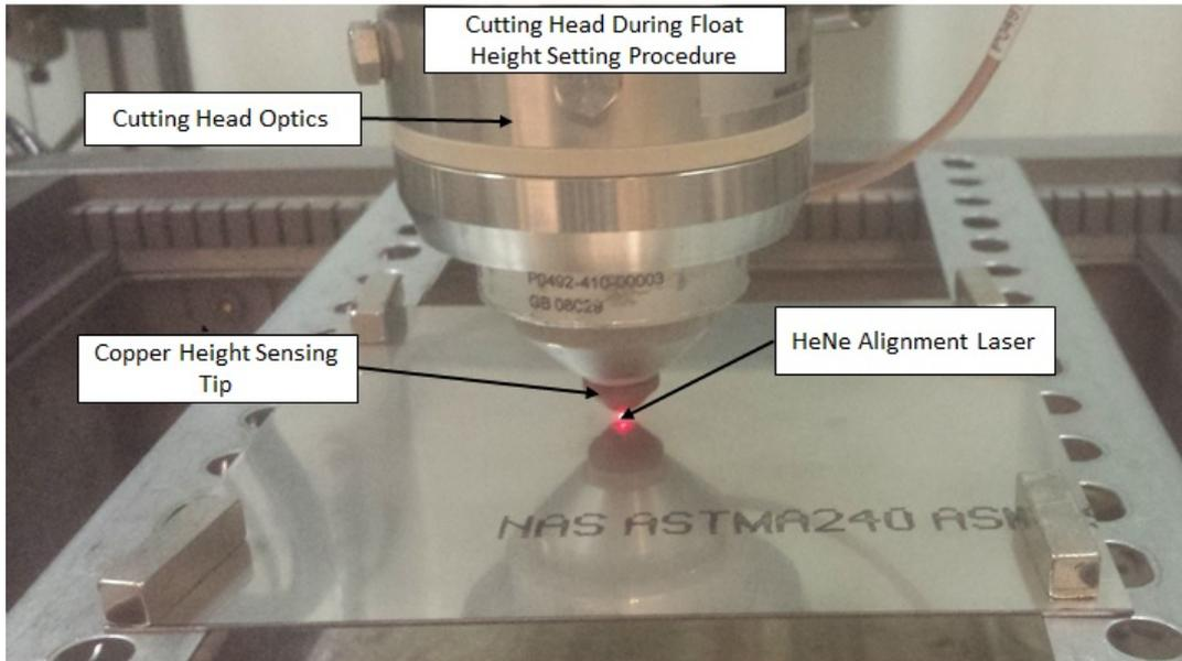
Figure 26: Initial step of cutting head height setting process.
