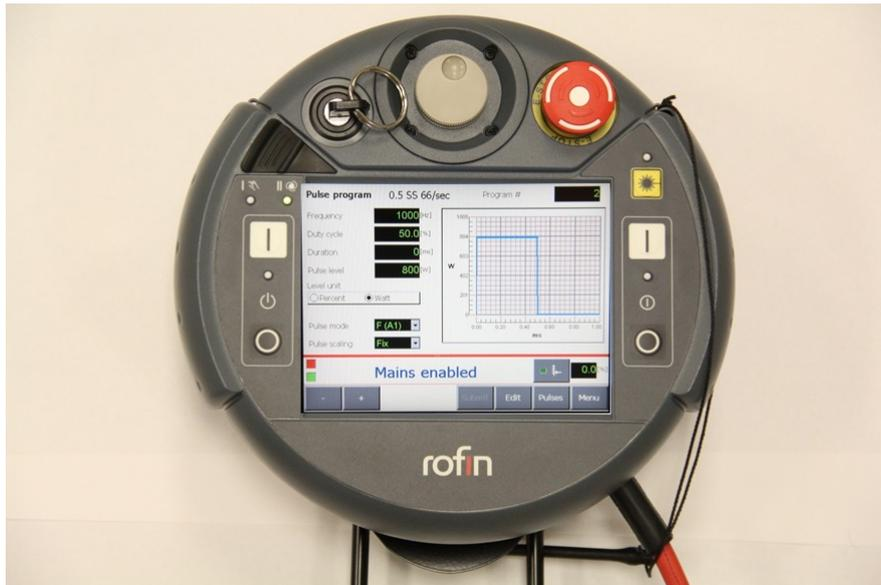
Figure 41: This screen shows all program parameters. To edit a parameter, select **Edit**. fields that can be changed will be highlighted in orange. To cancel changes, select **Cancel**.
