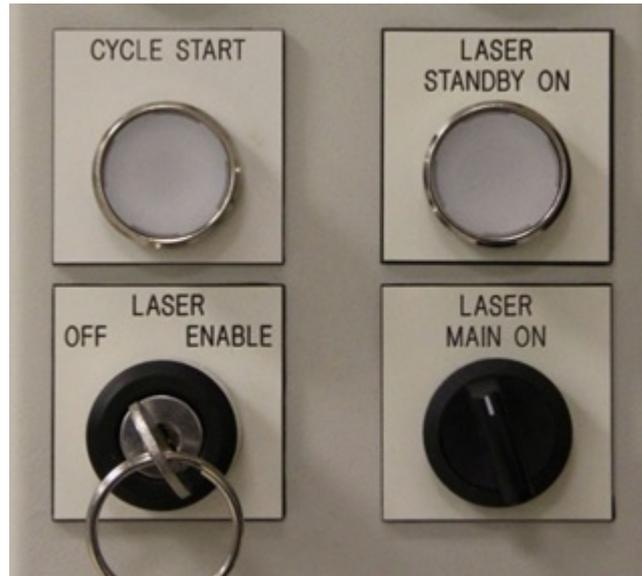
Figure 20: Lower portion of the workstation front control panel. These buttons/switches control the laser status.
