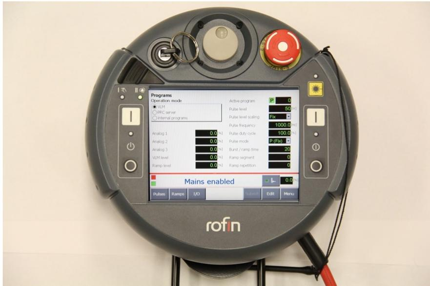
Figure 39: This screen provides an overview of the active program selected and allows one to access the pulse and ramp program lists. The upper-left box displays the current **Operation mode**.
