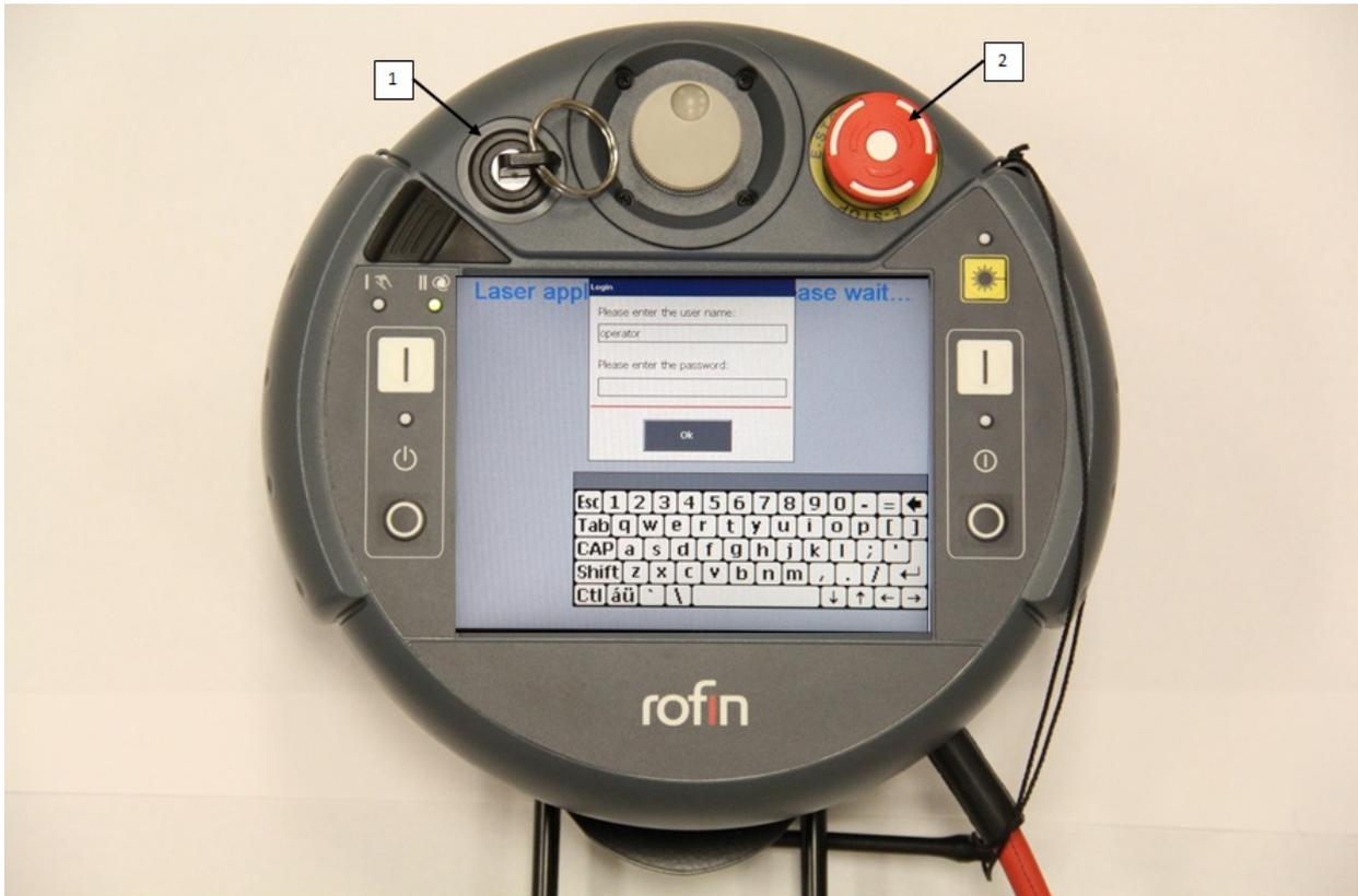
Figure 9: Laser source pendent log in screen. 1. Laser source control key, 2. Laser source E-Stop button.
