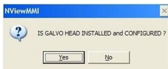
Check to ensure the galvo head is properly installed by checking for the presence of a data cable attached to the top of the galvo head. If it is installed click **YES**, otherwise shut down the system, install the galvo head data cable, and then select **YES**.
