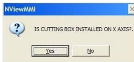
Check to ensure the cutting box is installed. If it is installed click **YES**, otherwise install the cutting box and then select **YES**.
