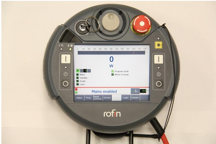
Figure 37: The Menu screen is the main navigation screen on the pendent and is the first to display after login. It provides simple details about the program mode, active program, and laser status. This screen also provides a real-time readout of laser power when the beam is on.
