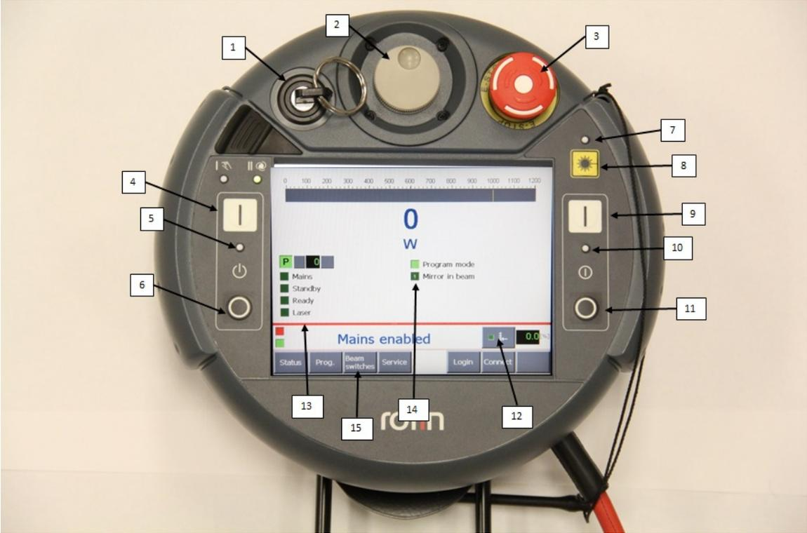
Figure 45: Pendent features for manual mode operation
