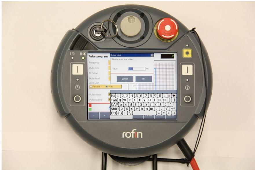
Figure 43: In the pop-up window Type in the desired value for that field and select **Ok**. **IMPORTANT: NO CHANGES ARE MADE TO THE PROGRAM VALUES UNTIL "SUBMIT" IS SELECTED!!**. To cancel changes, select **Cancel**.
