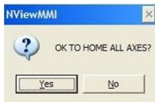
The third prompt will request to initialize and home the three axes. *Open the workstation door and inspect for/remove any obstructions that will impede axes motion. The x-y axes home in the far left corner of the work area.* If no obstructions present, close the door and select **YES** to home the axes. The Z-axis will home first, followed by the Y-axis and finally the X-axis.
