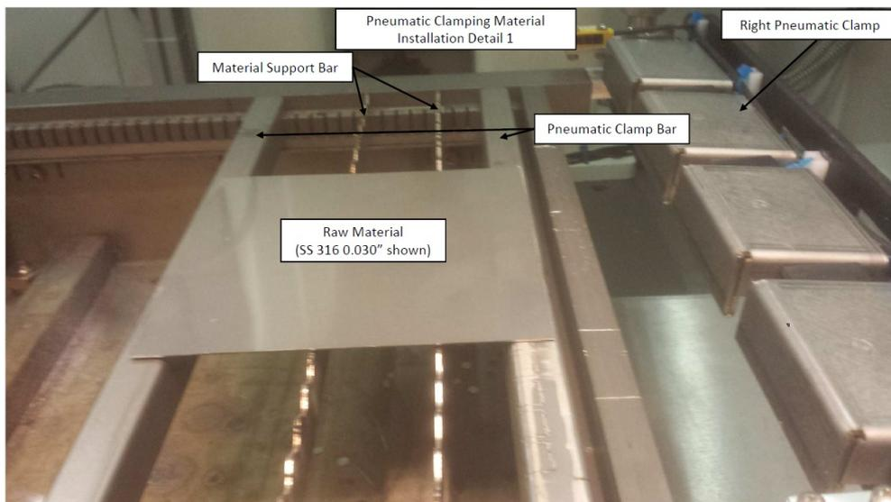
Figure 23: For **pneumatic workholding**, move the **pneumatic clamp bars** to fit the raw material size, ensuring there is sufficient overlap for the clamps to grip the material. add **material support bars** in the middle of the material to prevent excessive deflection from the assist gas pressure. Use as few as possible to prevent excessive wear on these consumable parts.
