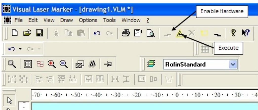
Figure 32: Top toolbar of the VLM software showing the **Enable Hardware** and **Execute** buttons.
