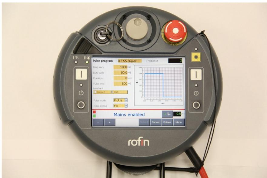
Figure 42: Select the field you wish to edit by tapping on the highlighted field. For applicable fields, a pop-up window will appear with a touch keyboard.
