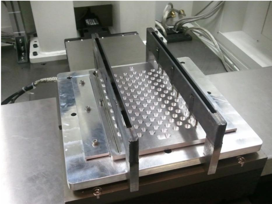
Figure 33: An example of fixed mode workholding for a large, 9x7[in] multilayered device. This setup includes a base plate datum, welding clamps, welding plate, and bar clamps to provide pressure.
