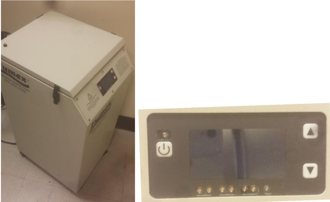
Figure 5: Rofin system fume extractor (left) and control panel (right).
