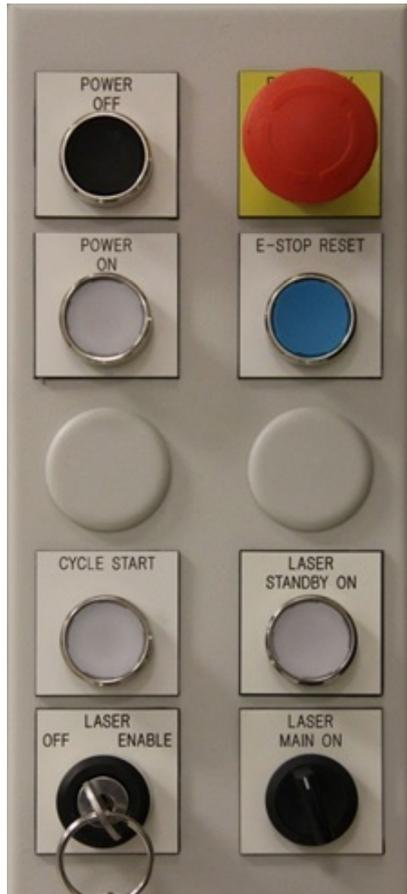
Figure 8: Workstation front control panel.
