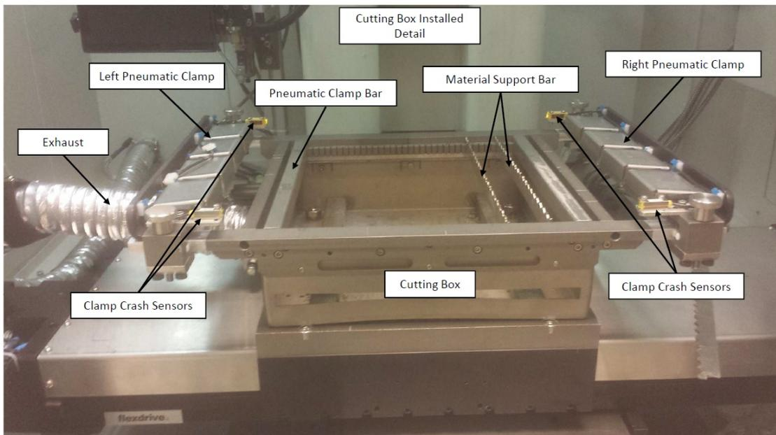
Figure 22: Cutting Box Parts.
