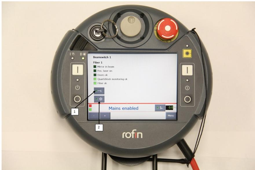
Figure 46: The Beam Switches page on the laser source pendent. 1. **Laser Select** button, 2. **HeNe Laser** button.
