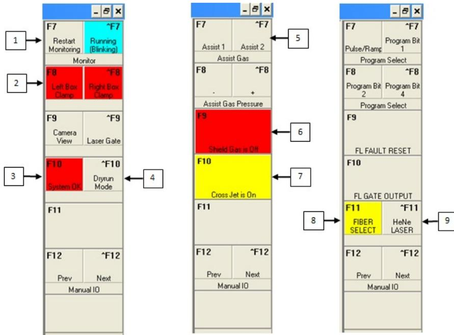
Figure 49: Additional F7 options menus available by navigating with the **F12** and **Ĥ12** buttons.
