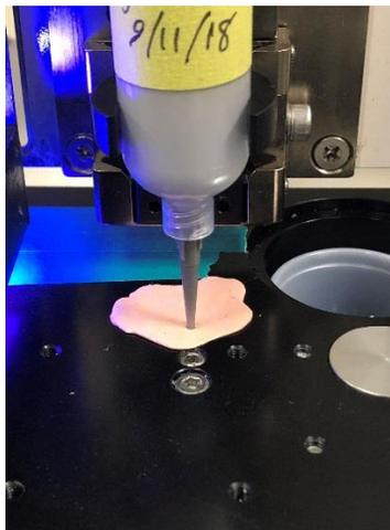
8. On the “Align camera on needle mark and press [Teach]” window, move the dispenser stage until the cursor on the camera screen lies in the center of the mark on the silly putty made by the nozzle, Then press “Teach”.
