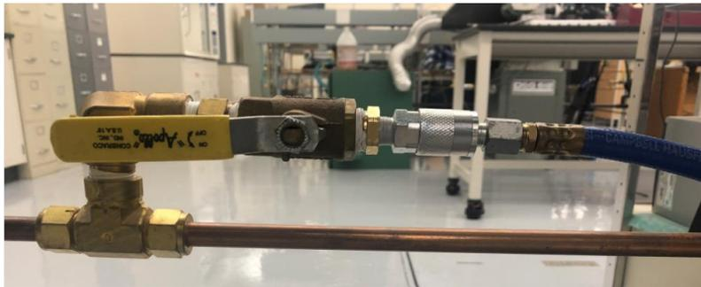
2. Ensure that the in-line air dryer is all the way open
